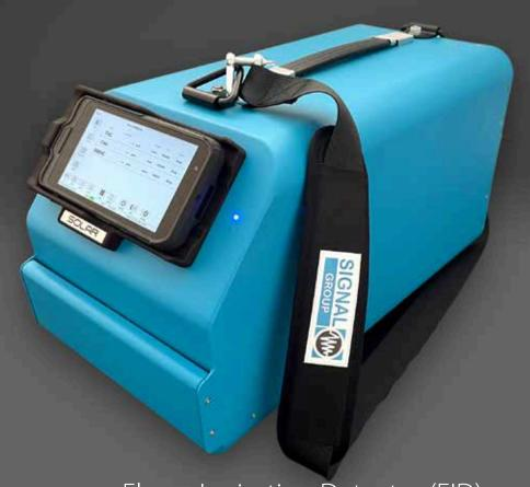
Flame Ionisation Detector (FID) analysers for the discontinuous measurement of the mass concentration of gaseous and vaporous organic substances in stationary source emissions.
