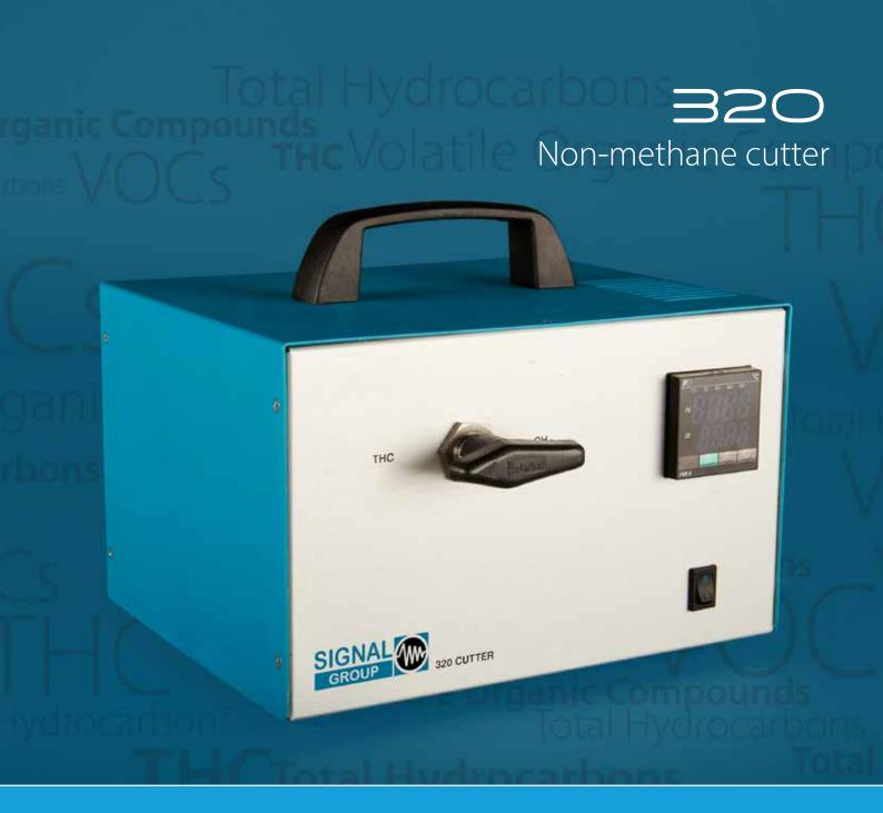
An external non-methane hydrocarbon cutter provides capability to measure methane only for clients with a standard heated flame ionisation detector (FID).
